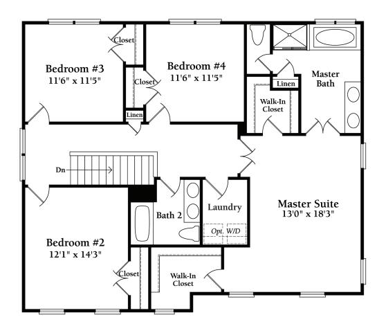
Upper Level Standard Floor Plan *Elevation A*
